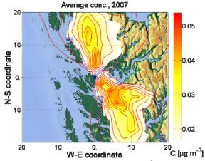
**Figure 2:** Simulated yearly mean MEA concentration in air ( $\mu g/m^3$ ) given meteorological conditions of 2007 in the 40×40 km<sup>2</sup> domain around Mongstad (blue cross).
